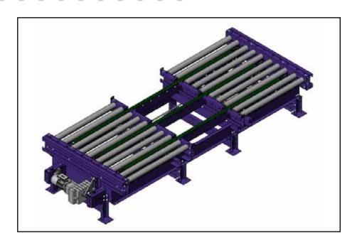
Double transfer modules combine the features and benefits of the roller systems and chain conveyor in one module. With a nominal roller pitch of 150 mm for all pallet types these transfers offer exceptional support for pallets during the transfer operation. The modules are available to suit the standard pallet conveyor widths.
