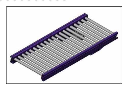
A robust pallet roller conveyor system. Rollers are driven tangentially by 5/8" chain in a fully enclosed side channel. The systems offers minimal backlash, easy tensioning and a 150/200mm roller pitch. With a load capacity of 1500kg per pallet the straight modules are available to handle upto 4500kg total conveyor load.
