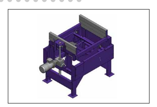
The beam lift assembly is designed to lift pallets 200mm above the chain conveyor. The beam assembly has two standard types, low and high. Low types range from 650mm to 800mm top of chain heights, high type beam lifts range from 850mm to 1000mm top of chain height.
