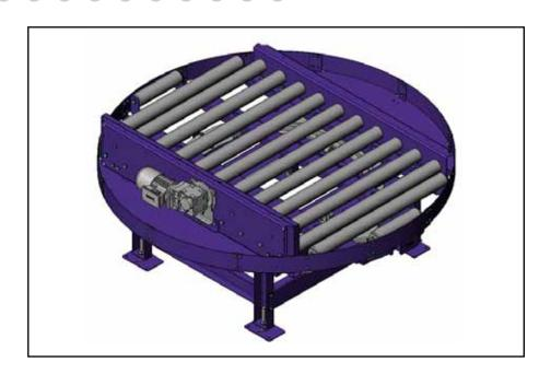
The turntable module is designed to change the direction of pallet travel by rotation of the pallet through any angle from 90° to 180°, whilst keeping the relationship of the pallet runners to roller conveyor the same.
