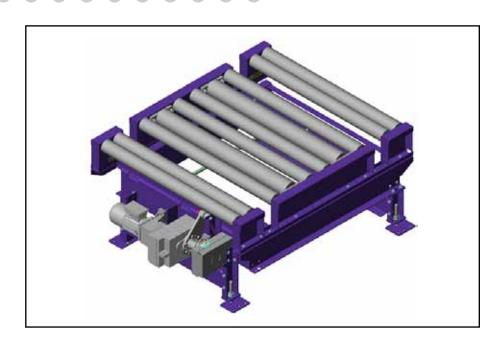
Roller transfers are a self contained unit, which can be fitted to a new or existing chain conveyor straight. The pop-up roller is powered by two motorised rollers. With a nominal roller pitch of 150mm for all pallet types these transfers offer exceptional support for pallets during the transfer operation.
