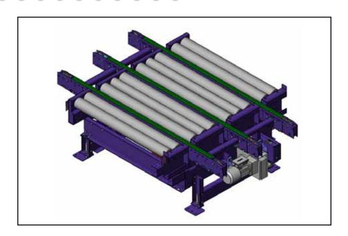
Centre transfer modules combine the features and benefits of the roller systems and chain conveyor in one module. With a nominal roller pitch of 150mm for all pallet types these transfers offer exceptional support for pallets during the transfer operation. Pallets can be received and transfered in either direction.
