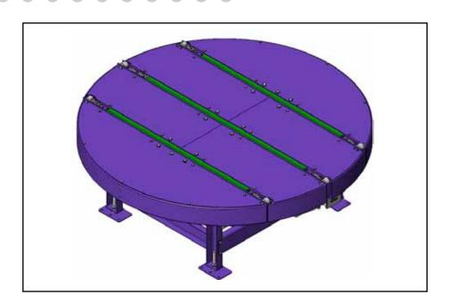
The chain turntable module is designed to change the direction of pallet travel by rotation of the pallet through any angle from 90° to 180°, whilst keeping the relationship of the pallet runners to roller conveyor the same.
