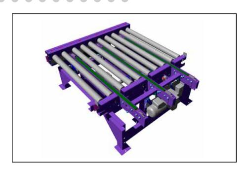
Transfer modules combine the features and benefits of the roller systems and chain conveyor in one module. With a nominal roller pitch of 150 mm for all pallet types these transfers offer exceptional support for pallets during the transfer operation.
