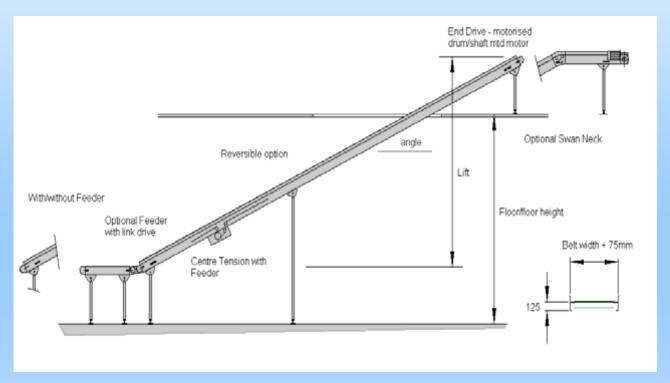
The Inclined Belt Conveyor range is part of **Riverbank Engineering** package handling solutions and utilise many common components.
