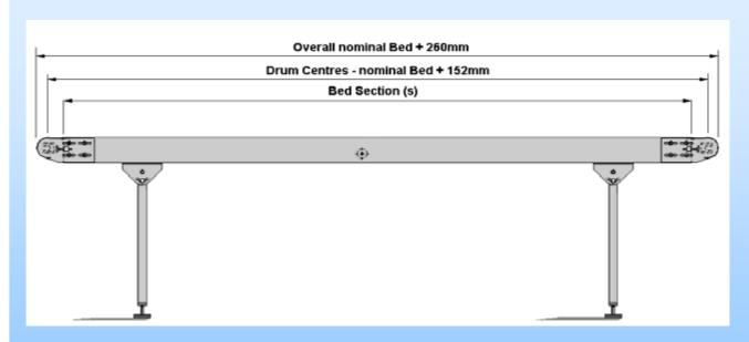
The Horizontal Belt Conveyor is designed to handle goods of various types. The standard version can be adapted with either a flat skid base, dished, troughed or with a roller base for heavier loads. This makes the Belt Conveyor a versatile option to suit your application and can be incorporated into a system with other types of conveyor.
