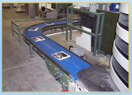
The flexible belting can take your product on one unit, round bends as well as inclines and declines with a continuous base and requiring only one drive unit, the modular belt conveyor is a more cost effective
