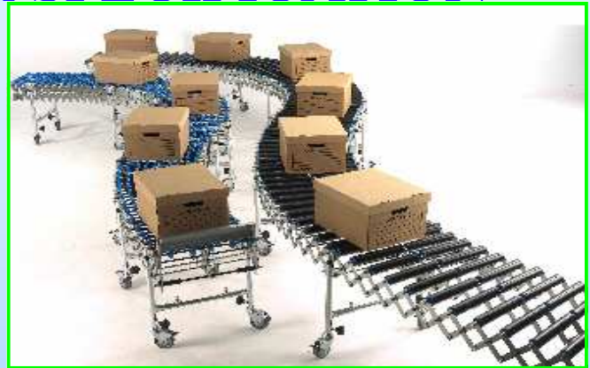
Skate wheels are ideal for tracking boxes around tight bends, rollers for general purpose use for handling products, packages or components with runners, rims or other uneven bases.
