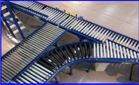
Lineshaft Conveyors showing straight track with a pusher and, from the bend, a merge unit.
